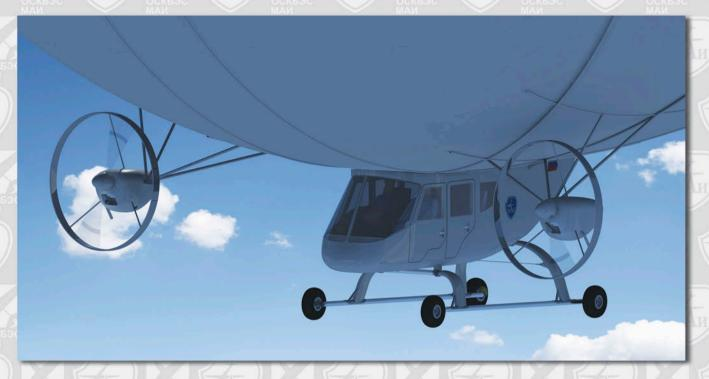
SkyBoat **HELIOS** uses aerostatic and aerodynamic lift in approximately equal degrees.
