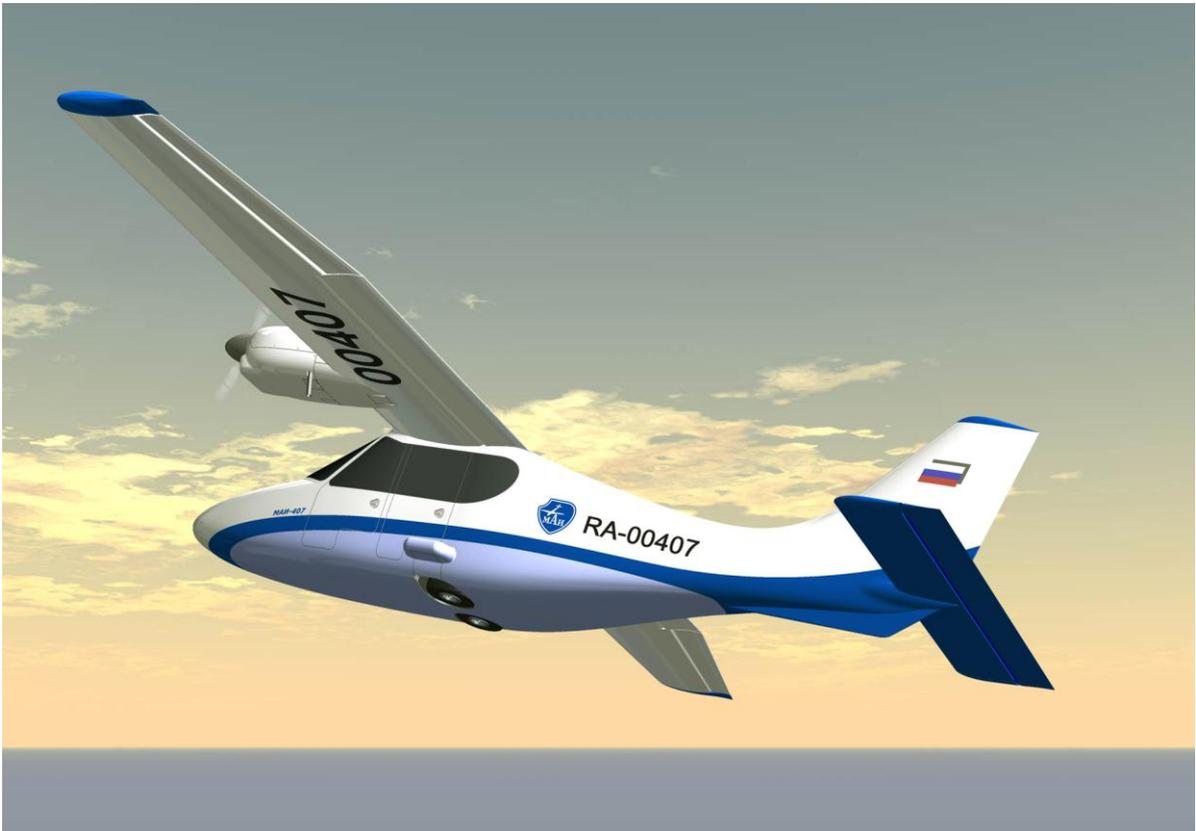
**MAI-407** multi-purpose four-seat twin engine airplane has been designed according to AP-23 Aviation Rule requirements, analog of European CS-23 and American FAR-23.
