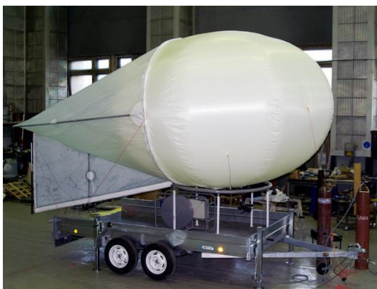
An example of use of the Colibris hybrid captive balloons is an aerostatic complex based on the K-15 balloon (15 m 3 ), intended for adjustment, parameters measurement and maintenance of radar stations
